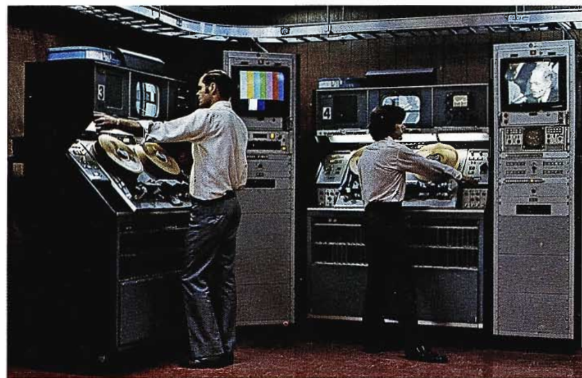
Master Control for Ch. 52 (left). (Right) Heavy tape production and program schedule keeps reels spinning on four TR-70 VTR's.
